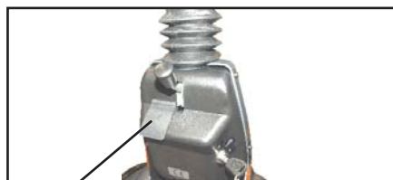
Connect the charging plug to the 3-pin socket on the steering column. The charging socket is located under the protective cover.
